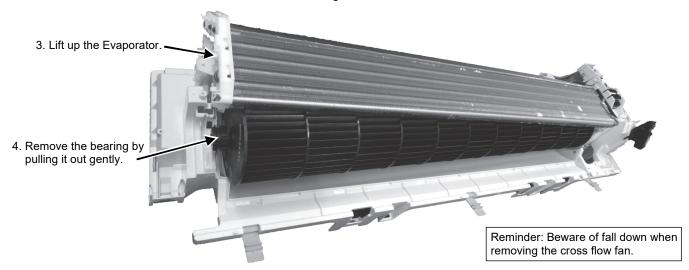
5. Remove the cross flow fan from the unit by pulling it to the left and downward.
